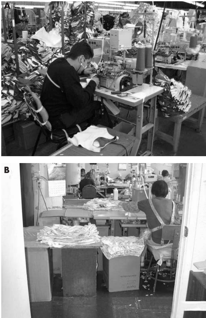
Figure 1 Typical sewing machine workstations; (A) operator leaning forward in a cramped space, (B) operator using non-adjustable household chair and cardboard boxes to support incoming fabric.
