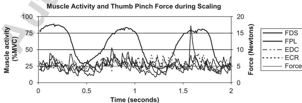
Fig. 3. Typical recording of muscle activity (RMS EMG) and thumb pinch force during scaling demonstrating approximately three strokes. The EMG spike is effectively filtered when calculating summary measures of peak force using the APDF 90%.
