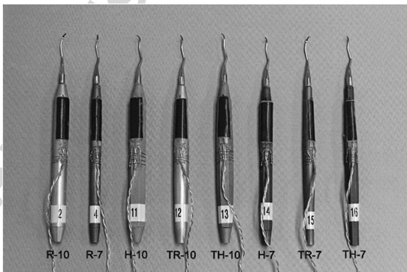
Fig. 1. The eight instruments used in the study are the same (e.g., surface texture, length, weight) except for cross-sectional shape. R = round; H = hexagonal; TR = tapered round; and TH = tapered hexagonal; 7 = 7 mm diameter; 10 = 10 mm diameter. The tool shape is symmetrical from the center to the ends. The force sensors are black.
