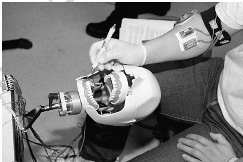
Fig. 2. Simulated dental scaling showing manikin positioned to simulate the clinical situation and surface electrodes attached to the right forearm of the subject. [Reprinted with permission from Dong et al. (2006), Copyright 2006 American Dental Association. All rights reserved.]
