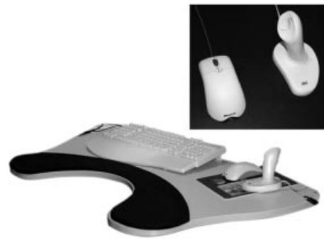
FIGURE 1. The study interventions were the padded forearm support board, the optical mouse (left; conventional) and the 3M mouse (right; alternative).
