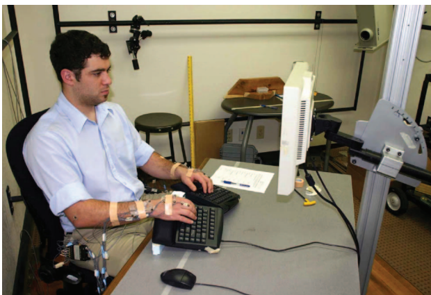
Figure 1. Experimental setup, subjects type during experiment while forearm and wrist postures are recorded by camera banks in the corners of the room.
