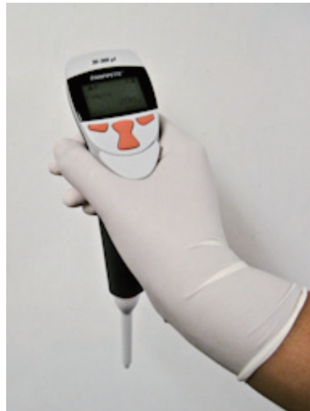
Fig. 3. Thermo Scientific FinnpiPETTE Novus held in hand.
