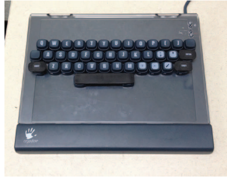
Figure 2. Keyboard with key spacing of 19 \times 19 mm.
