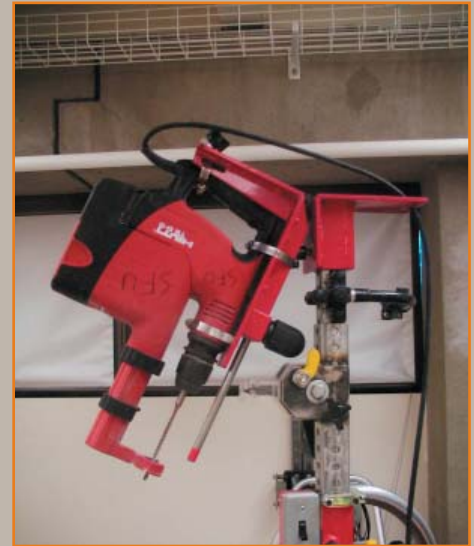
Hinged saddle to lower height
