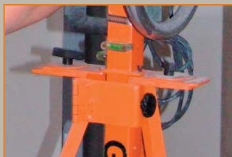
Column can be leveled to accommodate uneven surfaces
